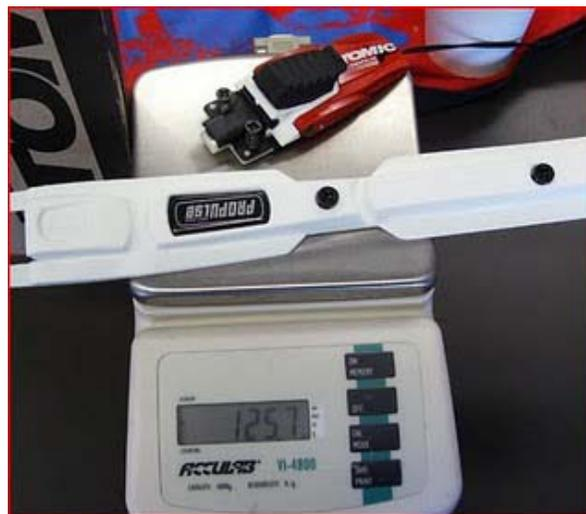
The new SNS Propulse has an improved rubber bumper that seems less likely to pop out of place over time, compared to the old Profil bindings. And the new latch mechanism is low profile, easy to grab, and also latches securely.
