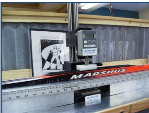
*Precise tools for measuring camber and flex.*
