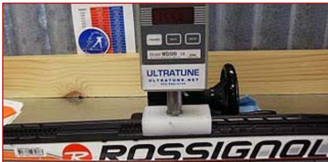
Also, the camber is slightly modified, with the half-weight camber open just a little further forward than the old WCS. The camber closes about another 10-12cm when progressing to full-weight, and this provides a great all-around front end camber, especially when combined with the somewhat more compliant tip flex than the old Xium.
